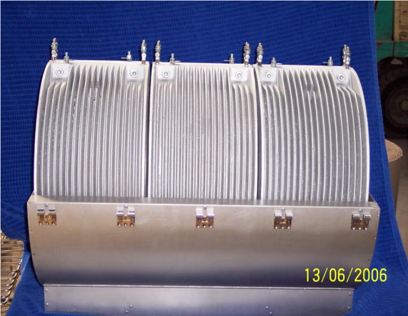
Finned heater assembly (top half of cowl removed)
